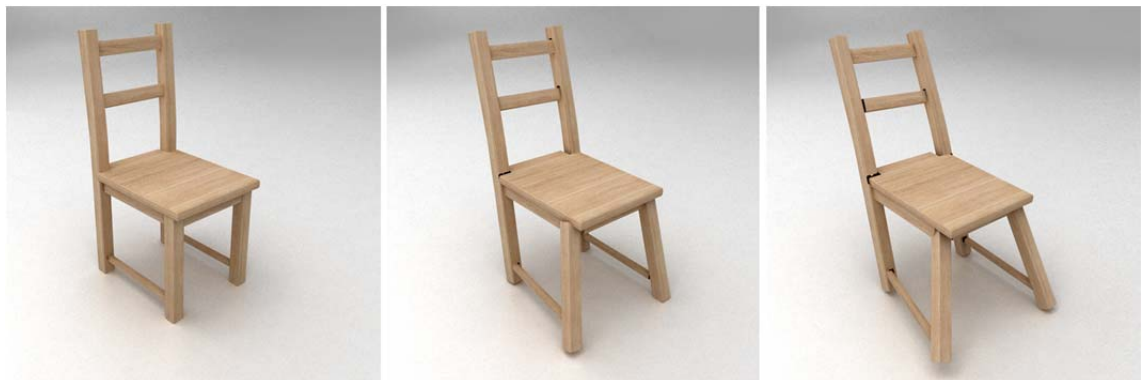
Fig. 11: Expected deformation. Simulation online: http://youtu.be/Lcaa00aK8yA
