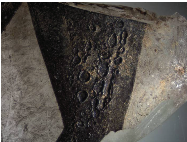
Fig. 3 -Optical micrograph in reflected light of the surface of sample KHV20; the black layer is affected by craters.
