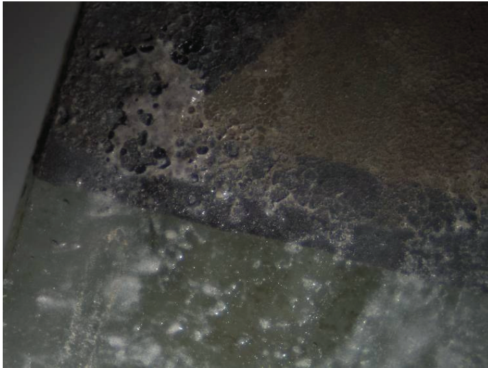
Fig. 4 - Optical micrograph in reflected light, sample HKV17. The white glass droplets deposited on the sheet glass surface (lower part of the micrograph) are in a good state of preservation, while the white glass deposited on the black layer is brittle and partly lost (flaking).
