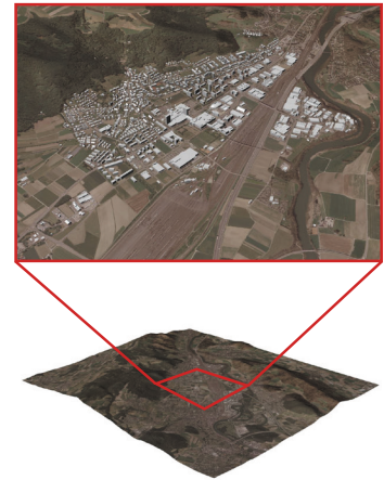
Figure 24: Generation of 3D topography including satellite imagery and 3D building geometries, in this case, Spreitenbach, agglomeration of Zurich, Switzerland. Source: Michael Walczak (2020)
