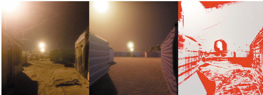
Figure 32: From left to right, actual photograph of the current light condition in Khayelitsha, Cape Town; simulated light conditions; and pixel comparison in red showing the difference between actual reality and simulated reality. Source: Photograph on the left, Stephanie Briers (2019); center and right images, Michael Walczak (2019)
