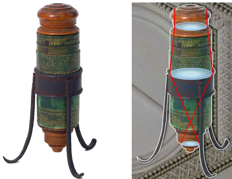
Figure 13. The “occhiolino”, designed first by Galileo Galilei (1624). The one on the image is believed to be of Giuseppe Campani. Credit: the Museo Galileo [83]. Adapted from [78].
