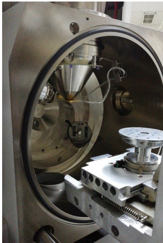
Figure 14. The sample chamber of a scanning electron microscope with the front door that holds the sample mount open. On the chamber top, the electron gun mechanism could be seen. (Taken at the electron microscopy lab of the Institute of Conservation, University of Applied Arts Vienna, April 2022.)
