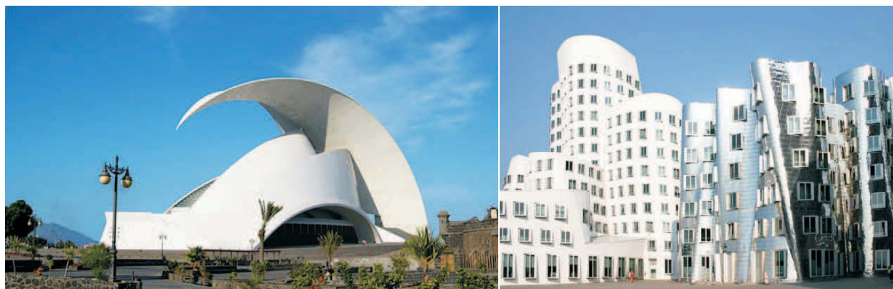
Figure 7. General cones and tangential developables in avantgarde architecture. Left: Santiago Calatrava's congress hall in Teneriffa shows parts of cones (©Santiago Calatrava, engineer and architect, reprinted with permission). Right: Frank O. Gehry works with general cones and tangential developables (Neuer Zollhof / Düsseldorf, ©Frank O. Gehry, reprinted with permission). Both architects use such surfaces in many of their buildings
