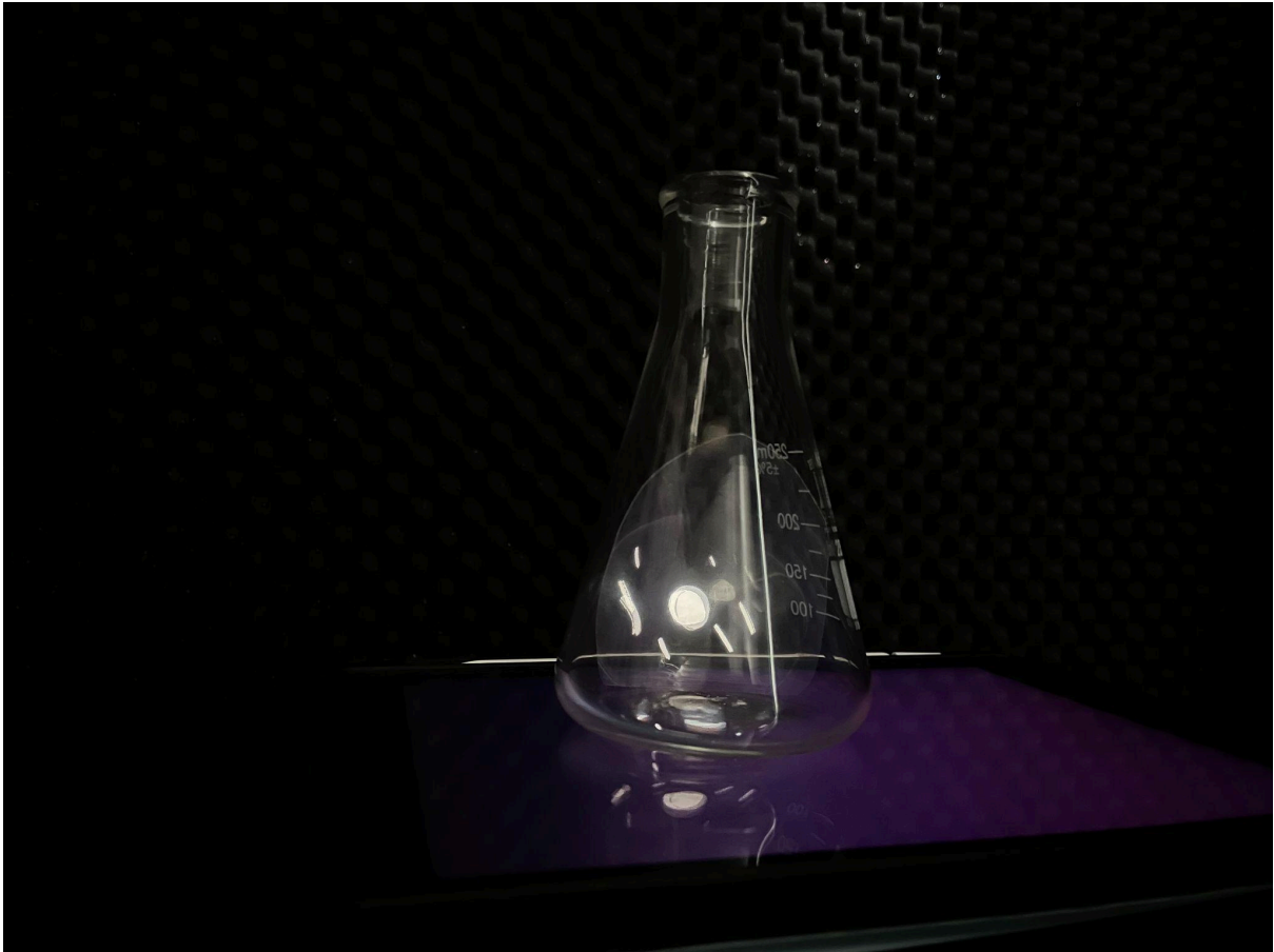
Figure 6. A Pepper's Ghost prototype using a chemistry beaker and transparent film. Photograph by the author, 2024.
