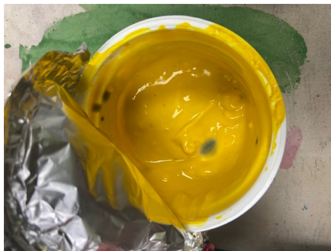
Figure 18: CI Pigment Yellow 180 based paint after 7 days of storage at room temperature, Copyright: Claus Schöning.
