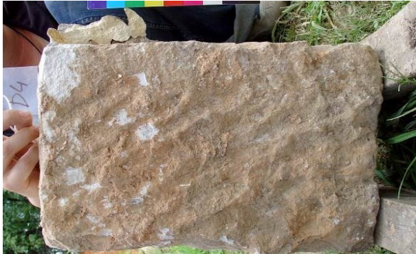
Fig. 3: Detail of processing with bolster
