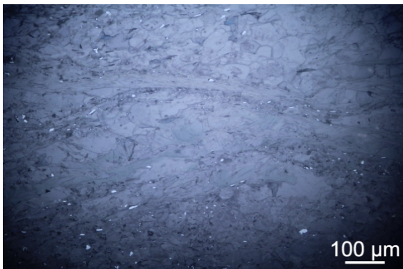
Fig. 21: Sample NEP_ST_1, Olympus BX40, incident light, bright field. Overview of mica inclusions (whitish spots).
