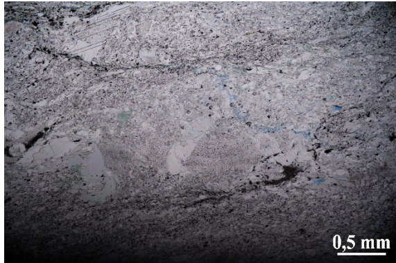
Fig. 19: Sample NEP_ST_1, Nikon SMZ 500, transmitted light, crossed polarizers. Overview of the rock matrix with coarser and finer layers.
