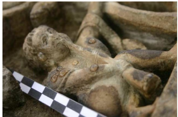
Fig. 15: Hydrophobic stone surface due to coating
