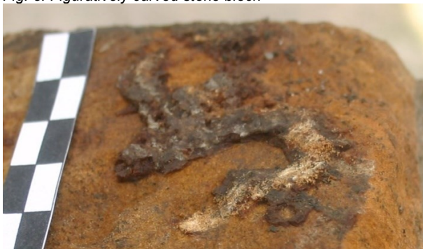
Fig. 7: Detail of copal glue used for fixing stone pieces (joints)
