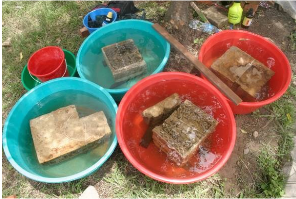
Fig. 16: Desalination within water bath with rainwater
