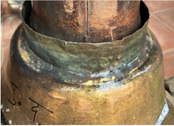
Fig. 9 and Fig. 10: Examples of corrosion: Dark brown copper oxide
