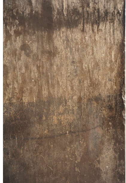
Fig. 12: Partial black crust on stone
