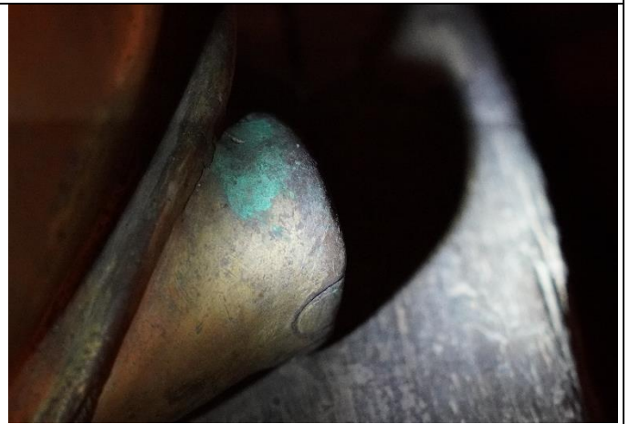
Fig. 6: Green corrosion on left hind leg of the right elephant (right lion)
