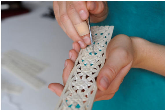
Fig. 26: Carving replicas for the reconstruction, 2017
