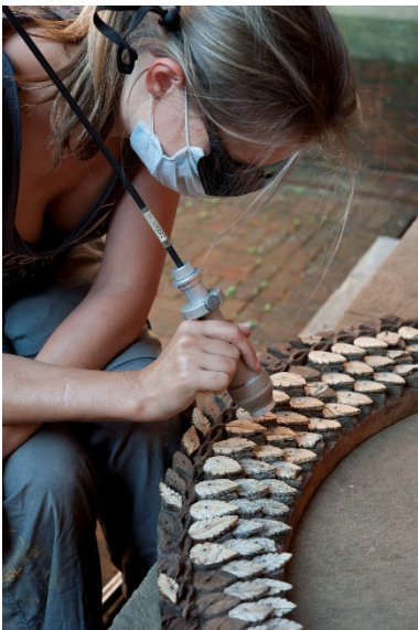
Fig. 19: Laser cleaning of the ivory parts, 2013
