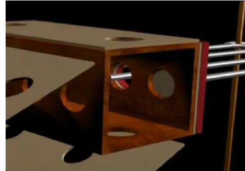
Figure 1: Jacquard loom: holes being "read" by pins
