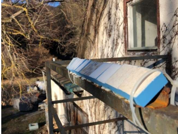
Fig. 31: first exposure of material sensors on a rack in Sattelbach, Lower Austria
