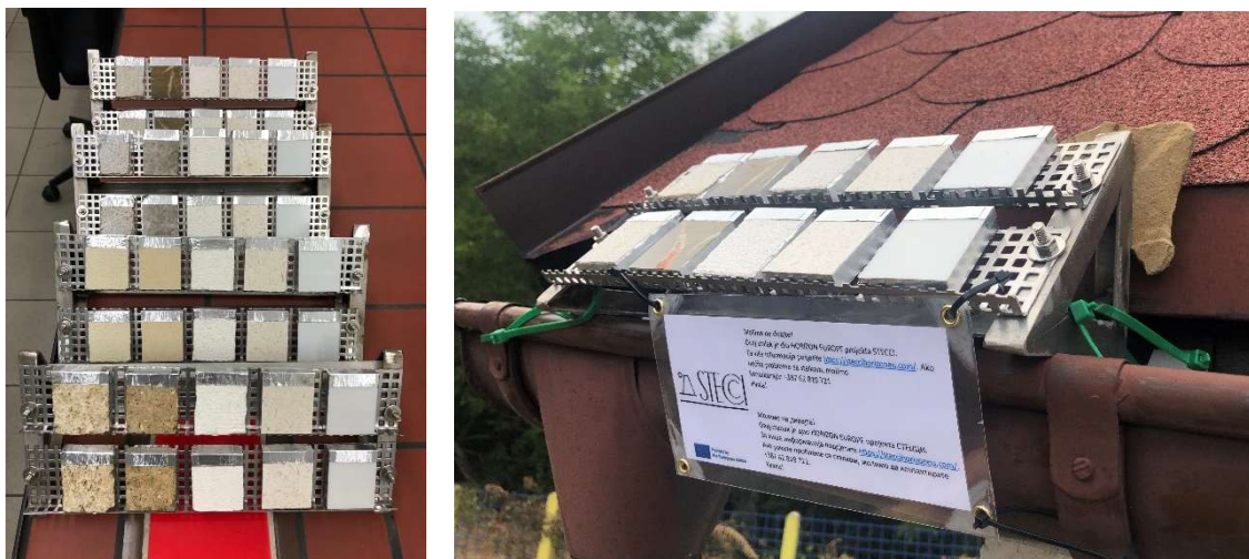
Fig. 44 and 45: The exposure racks for the STECCI project: four racks prepared for the installation (left) and the first installed rack (07.24) on the site of Kopošići in Bosnia and Herzegovina (right)
