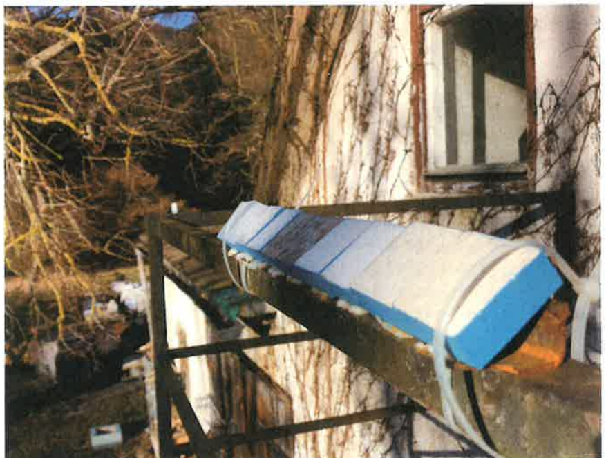
Abb. 1: Testreihe, exponierte mineralische Material-Sensoren (Marmor, Kalkstein und Alabaster) Fig. 1: Test series, exposed mineral material sensors (marble, limestone and alabaster)
