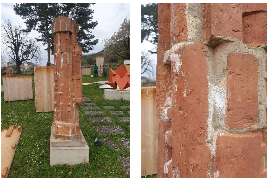
Fig. 72 and 73: Salt efflorescence visible after the dismantling of the winter shelters in spring, LEMU (© Katharina Breunhölter)
