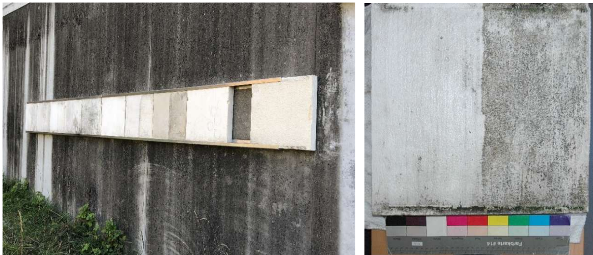
Fig. 78 and 79: Exposure of stone slabs with different shelter coats in Mauerbach, Lower Austria (left) and slab I (lime shelter coat) after 12 months of exposure, the right side of the slab is additionally treated with hydro repellent
