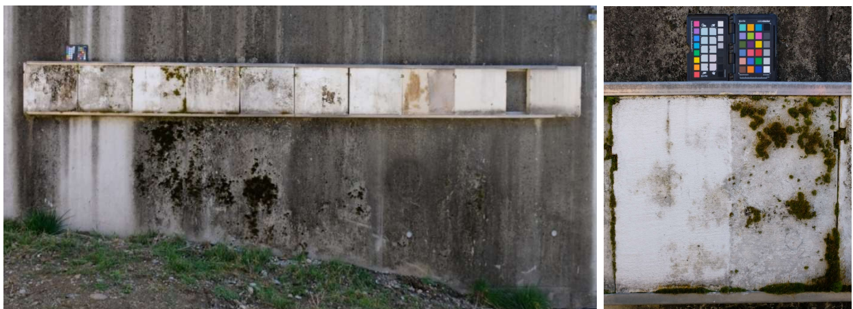
Fig. 80 and 81: after 8 years of exposure: stone slabs with different shelter coats (left) and slab III - lime shelter coat with white cement addition (right) (© Katharina Fuchs)
